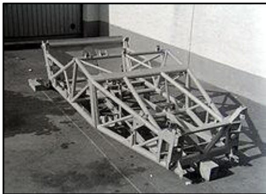
The C-Type's tubular chassis.
