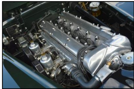
The Jaguar 3.4 liter twin cam engine
