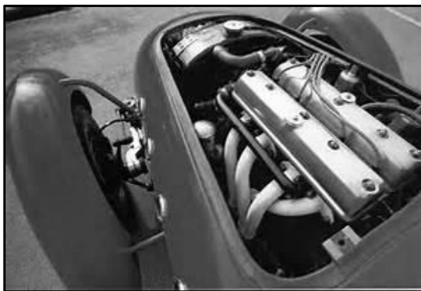
The Riley 2443cc engine
