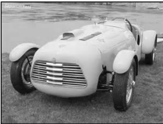
The completed body of the Barlow Simca 8 Special featuring the adopted Simca grill.
